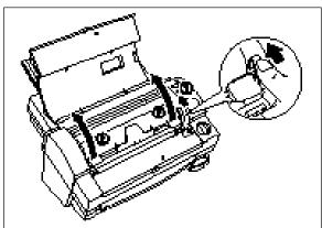
(2) Push the roller release lever (green color) and lift the roller holder upwards.
